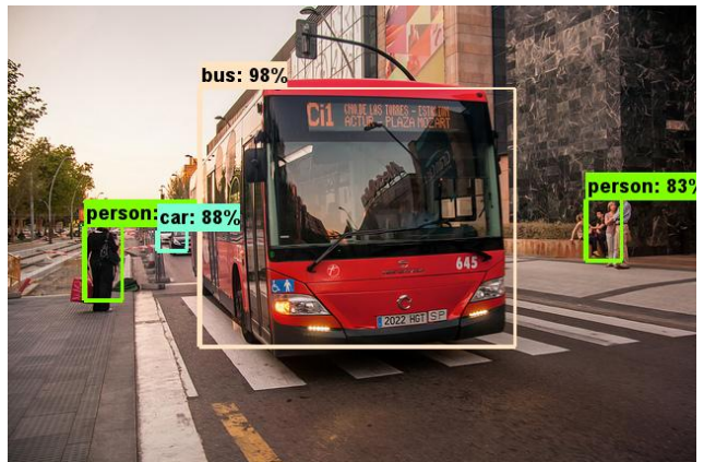
Figure 6. Example objection detection results using MobileNet SSD.
